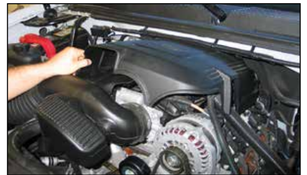
3. Lift up and remove the engine cover from the engine as shown.
